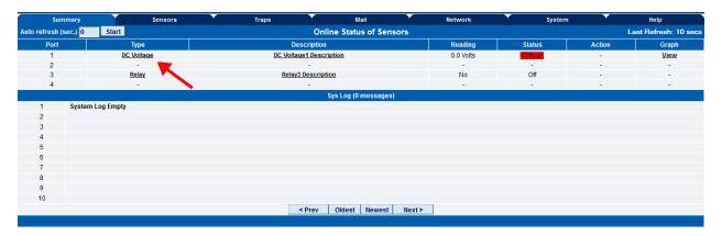
After logging into the base units web interface open the Summery page. The sensor will first be auto detected as the DC Voltage sensor and the status will be critical as shown in the screen shot above.
