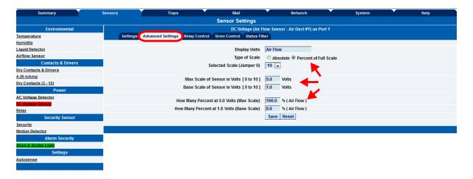
You can change the "Display Units" from Volts to Air Flow as shown above. Change the Type of Scale to Percent of Full Scale. Leave the Jumper setting at 10.
